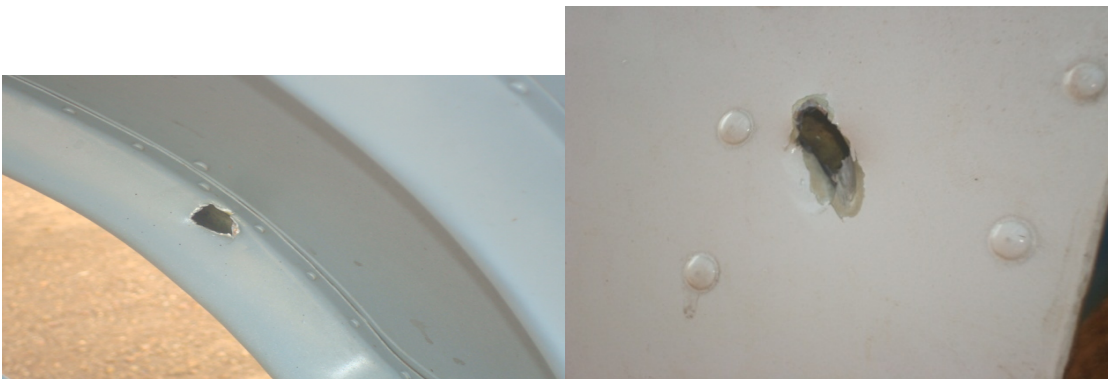
The bullet hole in the tire cover of helicopter UNO-883 (left), and in the left wing of helicopter UNO-881 (right).
